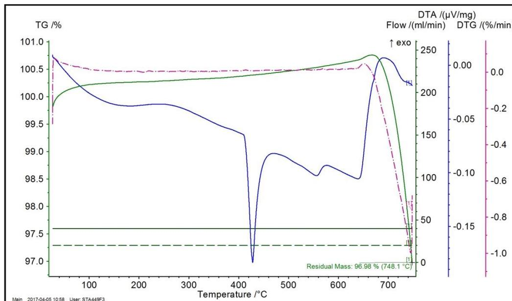
**Figure 3.** The result of the DTA analysis of hard zinc
