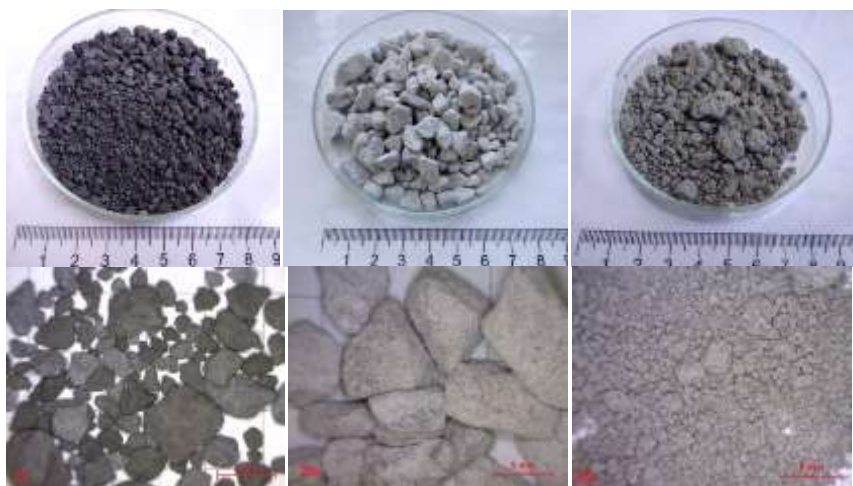
Fig. 2: Experimental slag samples: a) CHR1 - EAF slag (from carbon steel) CHR1; b) CHR2 - ferrochromium slag; c) and CHR3 - stainless steel slag
