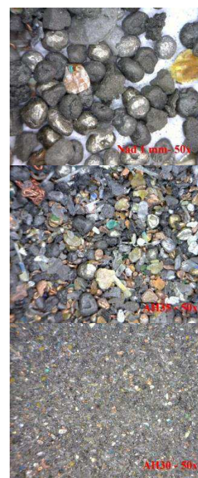
Figure 5. The influence of PCBs granularity on the accuracy of chemical analysis and particle fraction ( d \leq 2000 \mu\text{m} ), ( 1000 \leq d \leq 200 \mu\text{m} ) and ( d \leq 200 \mu\text{m} ) (50 zoom)
