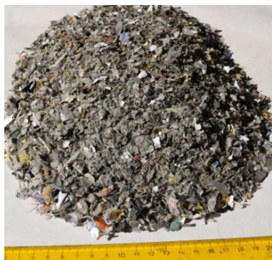
Fig. 2 Crushed PCBs of mobile phones—8 mm
