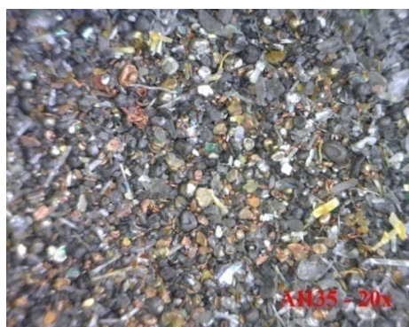
Fig. 5 Particle fraction ( d \leq 1 mm) (20 \times zoom)
