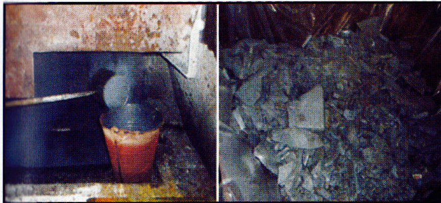
Fig. 3: Skimming the spent flux and flux skimming sample
