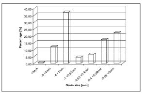
Fig.1: Histogram of crushed sample of LiA granularity.
