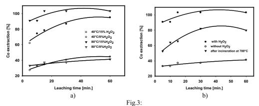
a) Kinetic curves of cobalt extraction in 2M sulphuric acid with and without addition of hydrogen peroxide at 40°C and 80°C (untreated sample), b) Kinetic curves of cobalt extraction in 2M sulphuric acid at 80°C with and without addition of hydrogen peroxide (untreated sample) and sample after incineration.
