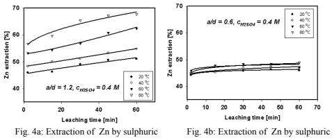
acid for a 20 g charge under various temperatures 70
