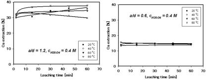
Fig. 8a: Extraction of Ca by sulphuric acid for a 10 g charge under various temperatures
