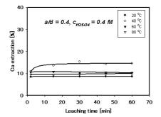
Fig. 8c: Extraction of Ca by sulphuric acid for a 30 g charge under various temperatures
