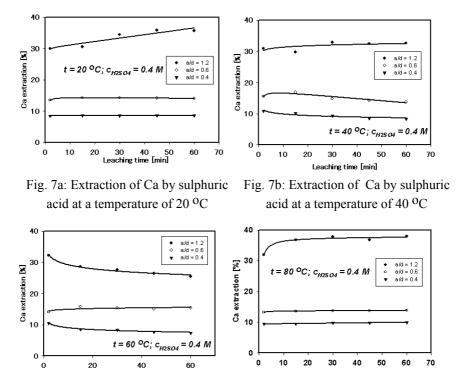
Fig. 7c: Extraction of Ca by sulphuric acid at a temperature of 60 °C
