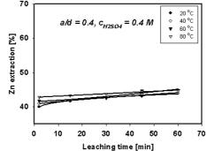
Fig. 4c: Extraction of Zn by sulphuric acid for a 30 g charge under various temperatures
