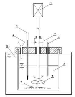
Fig. 2: Schematic view of the leaching apparatus 1 - stirrer engine; 2 - propeller; 3 - pulp; 4 - sampler; 5 - thermometer; 6 - feeder; 7 - water seal; 8 - water thermostat; 9 - EAF sample
