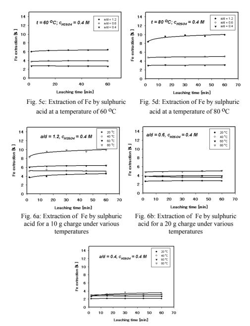
Fig. 6c: Extraction of Fe by sulphuric acid for a 30 g charge under various temperatures
